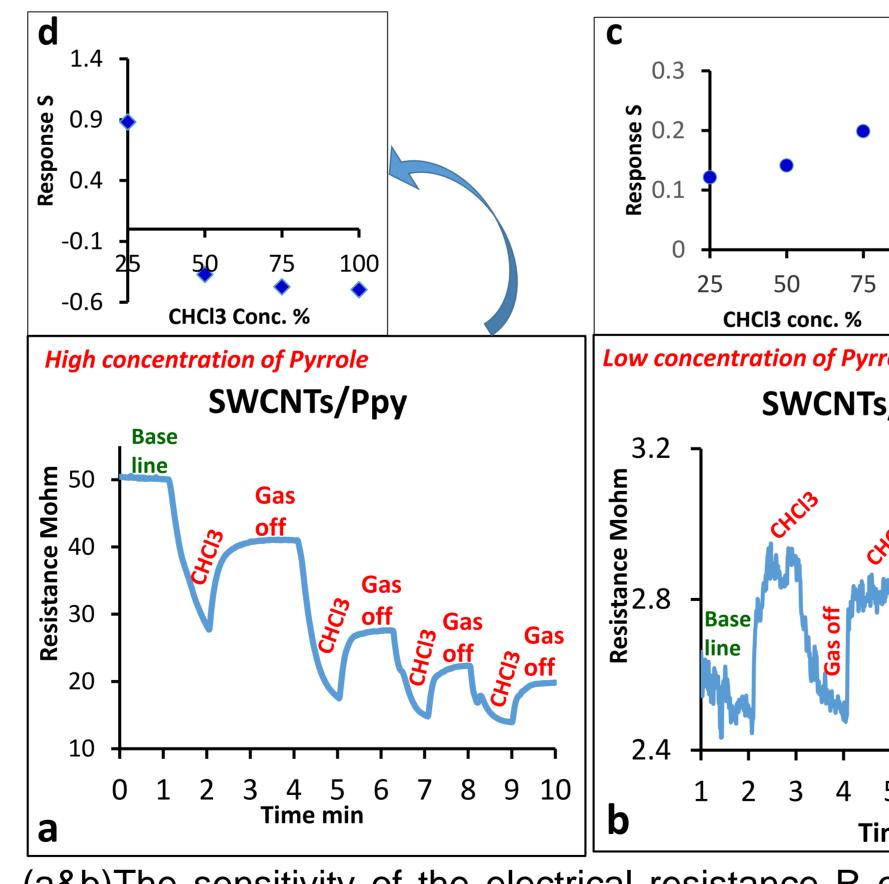
**Bare SWCNTs** 36.9 ш<sub>Ч</sub>о 36.85 75 100 Low concentration of Pyrrole 36.8 SWCNTs/Ppy 36.75 36.7 200 300 Time sec The sensitivity of the electrical resistance R of SWCNTs films to chloroform (0-100)% exposure at 17ºC. Time mir (a&b)The sensitivity of the electrical resistance R of SWCNTs/Ppy films to chloroform (0-100) % exposure at 17°C; (c&d) The device sensitivity S=(R-R0)/R0 as a function of chloroform. Fig (a) shows the swelling effect of pyrrole on the gas response.
