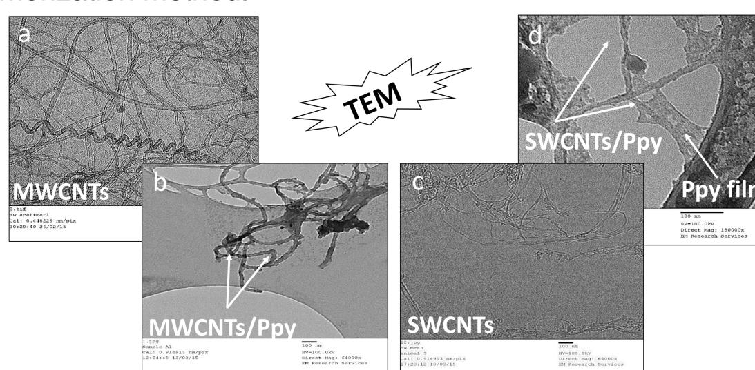
TEM images of (a) multiwall carbon nanotubes before coated by Ppy (Mag 130000x), (b) hybrid MWCNTs (Mag 64000x), (c) bare SWCNTs (Mag64000x), (d) SWCNTs after tamplated by Ppy (Mag1800000x).
