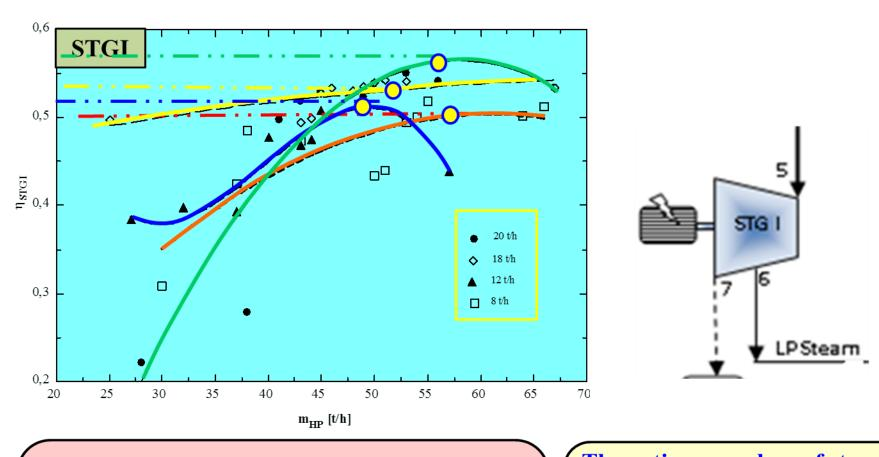
The exergy efficiency increases with HP mass flow rate to reach maximum values as follows: 50 % for condensation flow rates of 8t/h 51% for condensation flow rates of 12t/h 56 % for condensation flow rates of 20 t/h
