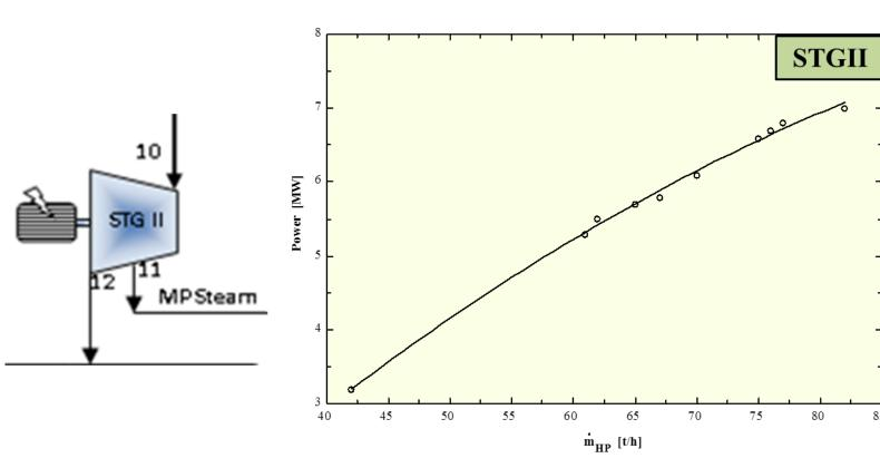
For the back pressure steam turbine STGII, The generated power increases linearly to achieve about 7 MW for a HP steam mass flow rate of about 82 t/h.
