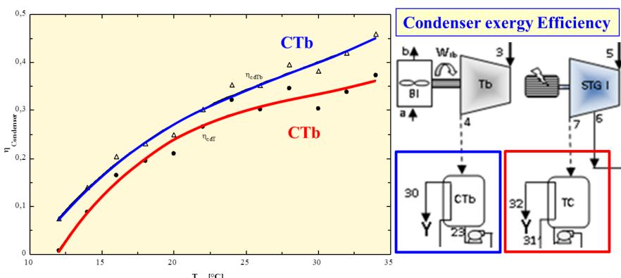
Increasing the seawater temperature from 12 to 24 °C leads to an increase of the exergy efficiency of about 6 times for the turbo blower condenser CTb and 14 times for the turbine condenser TC.
