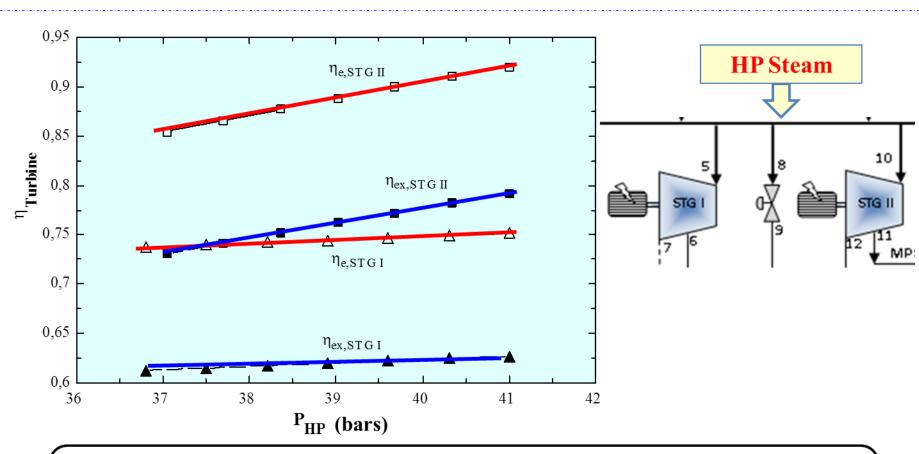
The energy and exergy efficiencies increase linearly with the pressure of steam. For the explored ranges of pressure, the energy efficiencies increase of about 1.37 % and 8.8 % for STGI and STGII respectively.
