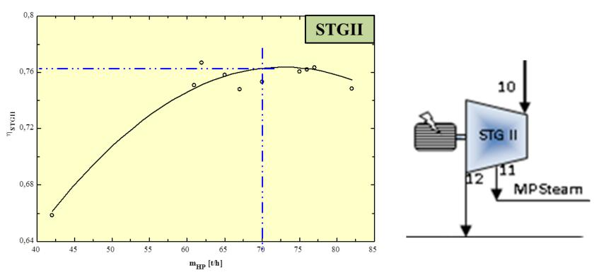
The exergetic efficiency increases sensibly with HP steam mass flow rate to reach a maximum value of about 75.5 % for a mass flow rate of about 73 t/h. That can be considered as an optimum value for the STGII supply.
