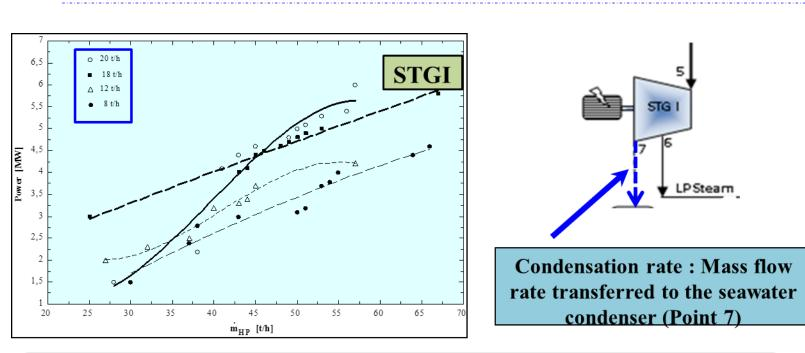
The generated power increases gradually with HP steam mass flow rate. For HP steam flow rate less than 35 t/h the generated power in not significantly affected by the condensation rate.
