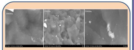
Fig.13 SEM analysis on the surfaces of the polypropylene resin with Kenaaf fiber shows the fine distribution of fiber in resin in matrix with the required resolutions.
