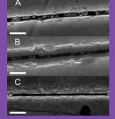
Picture 2 – SEM micrographs of 400 (A), 200 (B) and 100 © nm wide, contrasted with 252 nm gold NPs. Bar 1 um
