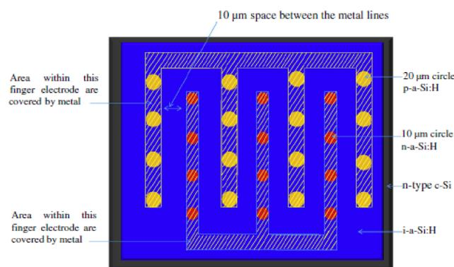
Fig. 2 Illustration of rear side geometry of the back heterojunction (a-Si:H/c-Si) solar cell. Here, p-type a-Si:H and n-type a-Si:H doped areas are shown as colored circles having diameter of 20 μm and 10 μm respectively<sup>2</sup>.
