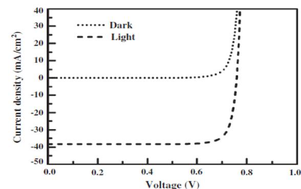
Fig.3 Dark and light I-V curves under forward bias.
