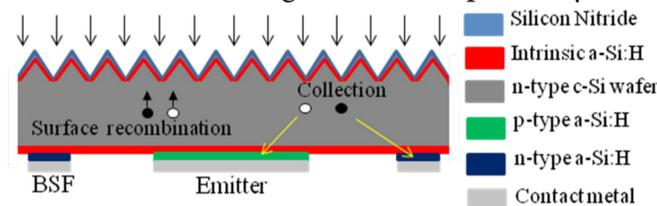
Fig. 1 Schematic cross-section of BHJ solar cell.
