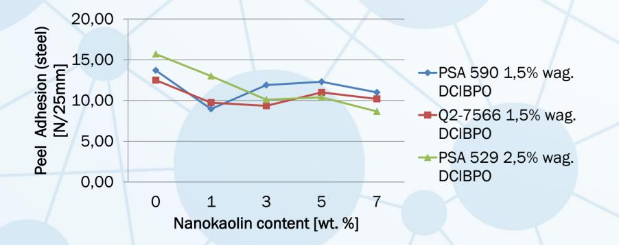
Fig.2 Adhesion of silicone PSA coutaining various amout of nanokaolin
