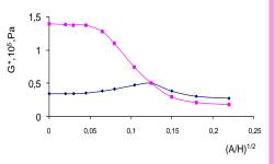
Fig. Real (red) and imaginary (blue) shear modulus of diethylene glycol
