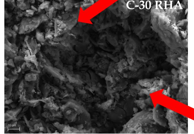
Compressive strength decreases with the addition of RHA, according to data from water absorption. High compressive strength for the fired bricks is achievable at the lowest levels (10 wt %) of the biomass fly ash (36 MPa).
