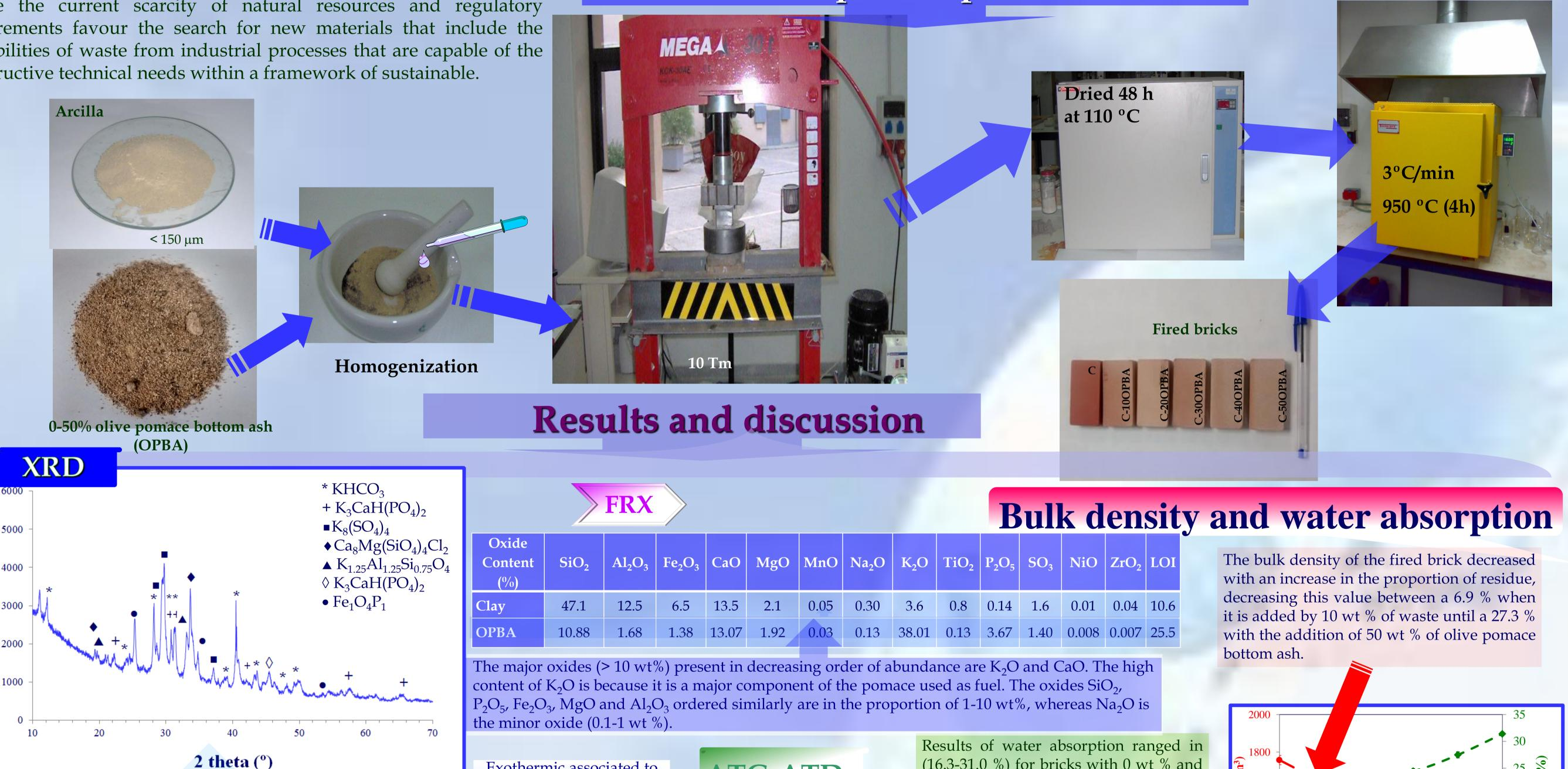
The mineralogical characterization of the olive pomace bottom ash showed the presence of an alkaline carbonate Exothermic associated to **ATG-ATD** combustion of organic matter and remaining unburnt maiter 42
