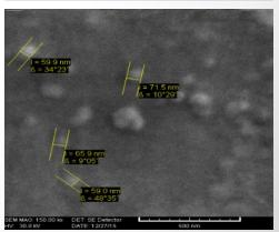
Fig. SEM image of prepared nanocapsules
