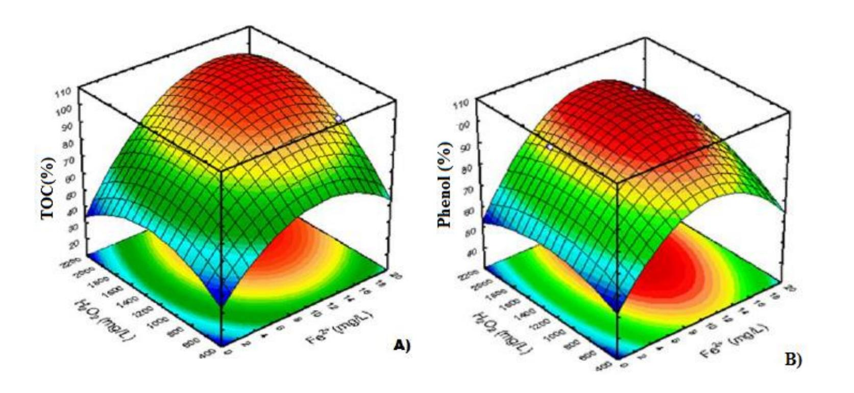
Figure 1: a) surface mineralization of phenol b) degradation of phenol applying photo-Fenton process.
