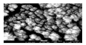
**Figure 1**: Nano gold aggregates on the surface of placer gold.
