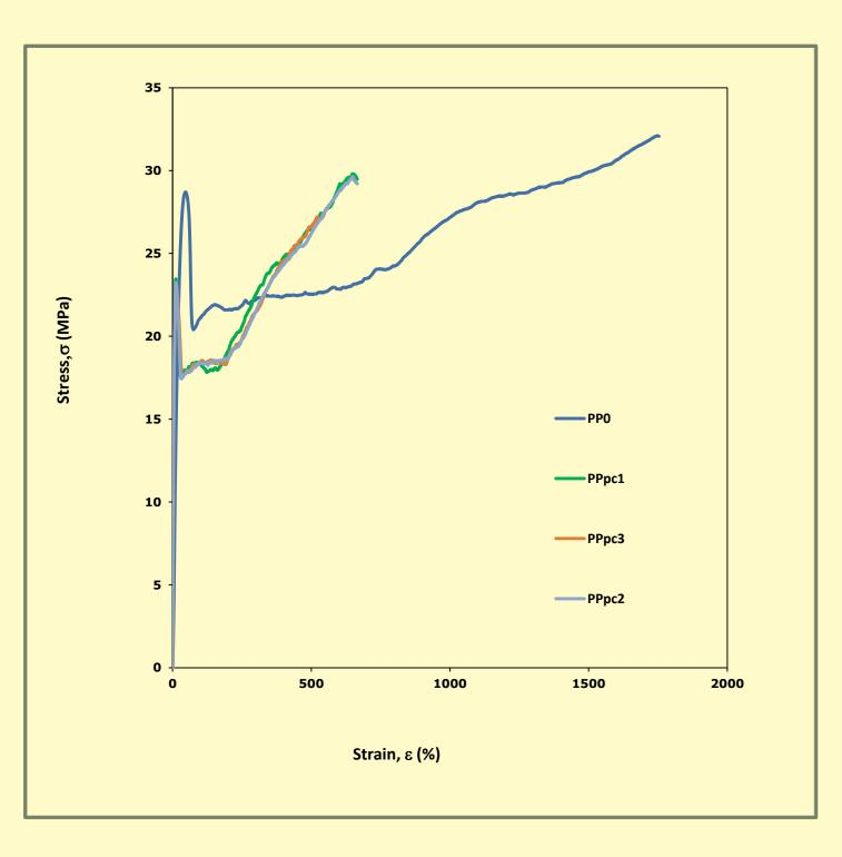
Most of the mechanical properties of the post-consumer polypropylene decrease after recycling compared to virgin polypropylene During simulated recycling the mechanical properties (elongation-at-break, yield stress and Young's Modulus) dropped initially and increased again upon second and third recycling cycle. However, impact strength showed opposite behavior.
