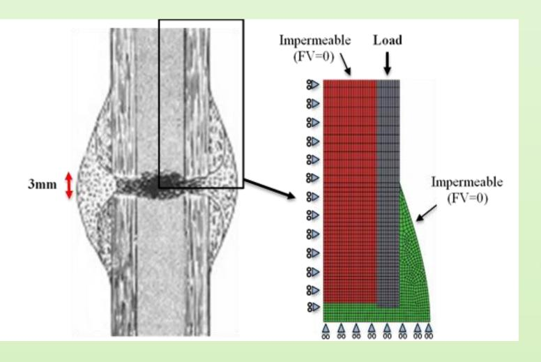
Figure 1: Axisymmetric FEM of a fracture ovine tibia with a 3mm fracture gap. Load applied at the end of cortical bone.
