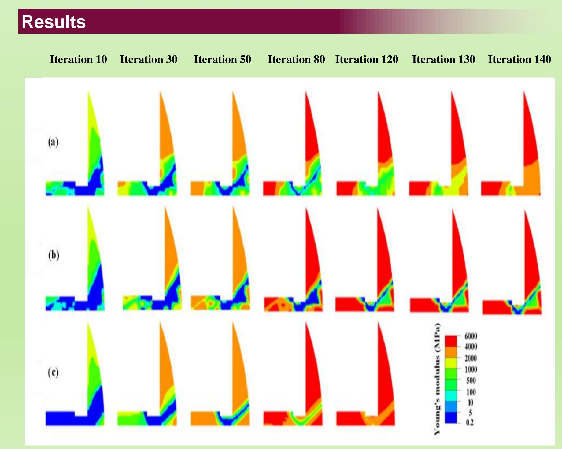
Figure 2: FEA results of fracture healing patterns for an external load of 500N. (a): using 1<sup>st</sup> model [1]; (b): using 2<sup>nd</sup> model [2]; (c): using 3<sup>rd</sup> model [4,5,6].
