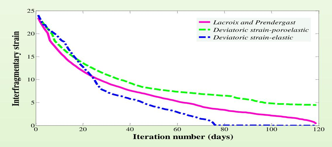
Figure 3: Interfragmentary strain for an external load of 300N. It can be seen that the interfragmentary strain for the 2<sup>nd</sup> model does not approach zero, which means that healing is not completed and leads to non-union.
