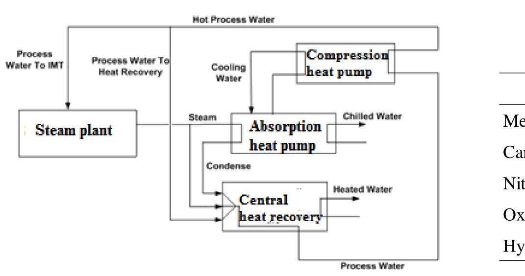
Figure 1. Scheme of the trigeneration system
