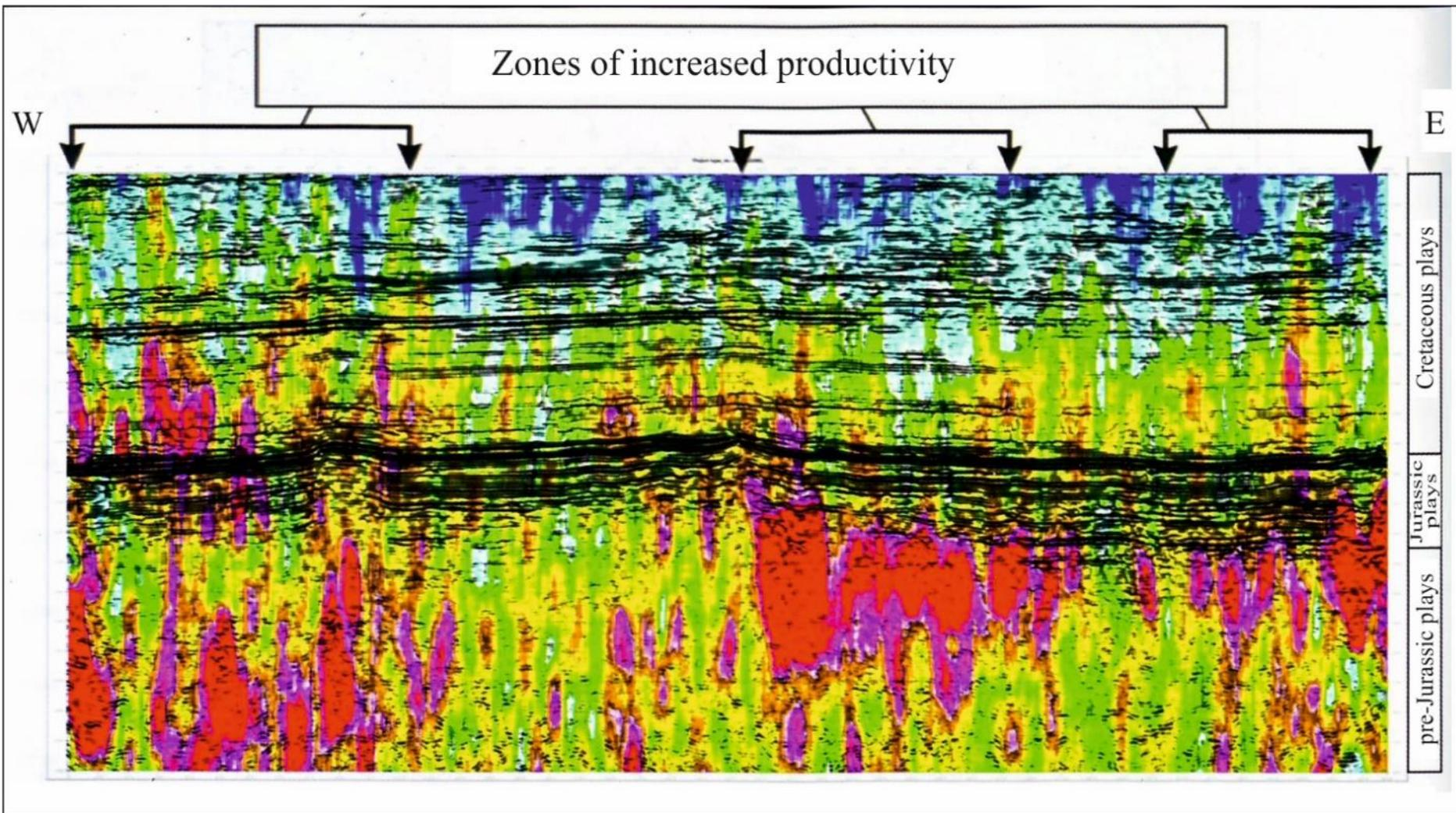
**Aganskoye field. Integrated time section of reflected and scattered wavefields. Red colours highlight the most disintegrated areas of the section—fluid-conductive structures.**
