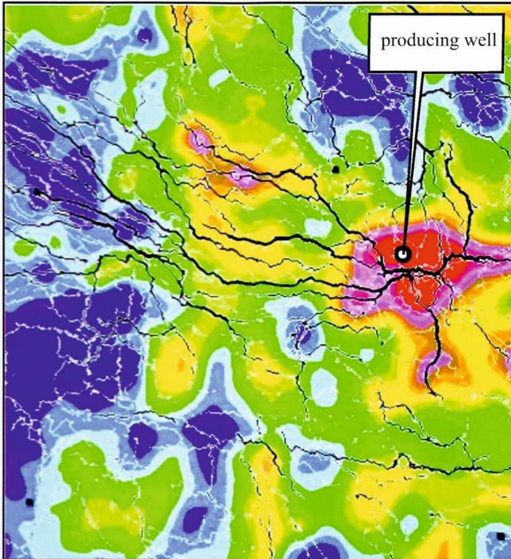
**A comprehensive characteristic of medium disintegration in the Bazhenov Formation interval (scattered wavefields and singularity (black lines) of seismic field). According to V.V. Charachinov et al., 2015**
