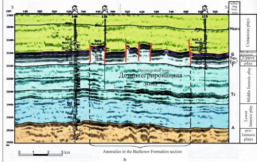
Shiromoye Priobye (Latitudinal Ob River Region). Vertical section of 3D seismic wavefield of one of petroleum fields:
