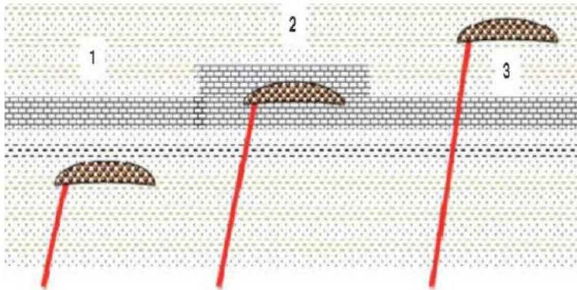
**Models of pools formation and structure of the Bazhenov Formation depending on the height of penetration of an echelon faulting from the basement into the sedimentary cover and depending on stratigraphic level of deep petroleum fluids discharge. According to Timurziev, 2015.**
