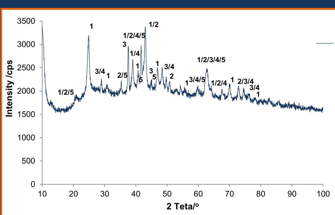
**Fig.1.** XRD pattern of naturally dehydrated deposits which have been scraped from beginning part of corroded steel pipe.
