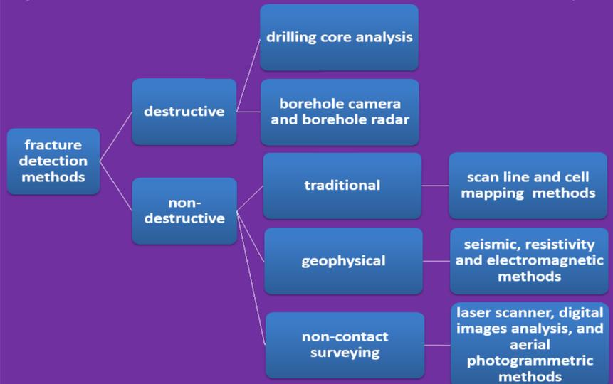
Fig. 2. A classification survey to fracture detection methods, see a sample from the surveyed publications in [1,2,3,6,7,9,10,11,12,13,14].
