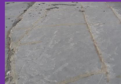
Fig. 3. Out-cropping large aperture vertical fractures in the bench surface.
